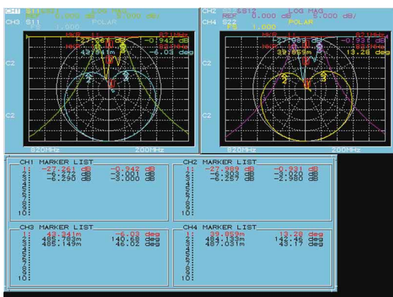
4-channel, 6-trace display with MARKER LIST SPLIT ON
